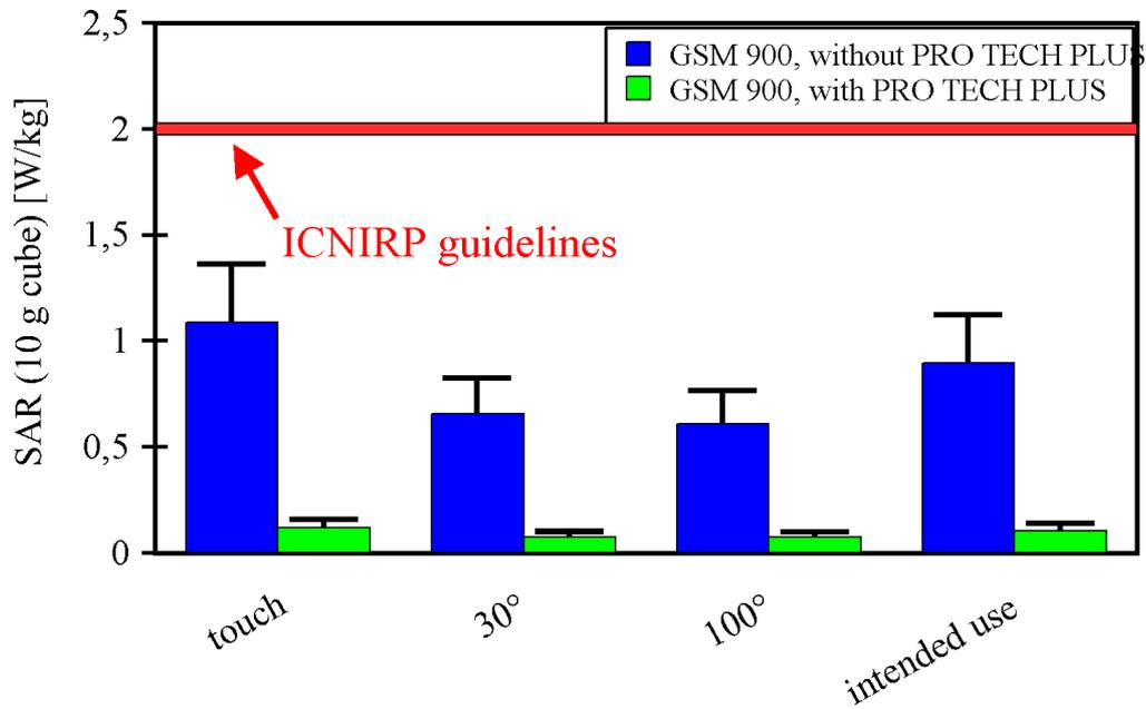
Fig. 8: The measured SAR values for GSM 900 using the Nokia 5110 in comparison to the ICNIRP Guidelines without and with the PRO TECH PLUS (left hand position).
