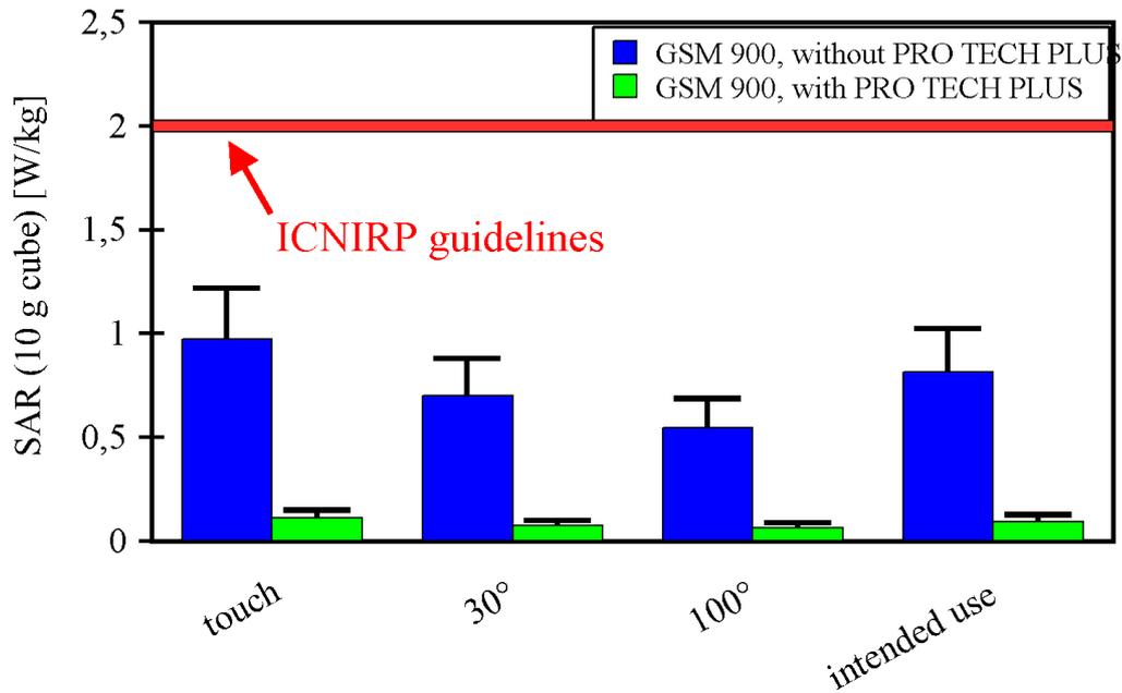
Fig. 9: The measured SAR values for GSM 900 using the Nokia 5110 in comparison to the ICNIRP Guidelines without and with the PRO TECH PLUS (right hand position).
